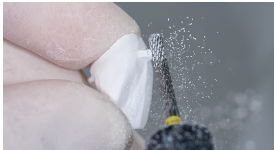
Fine tungsten carbide burs or diamond grinding instruments are recommended to smooth out the attachment points of the holding bars. Rough tungsten carbide burs and/or grinding instruments are not suitable, as they may cause chipping, among other things.
